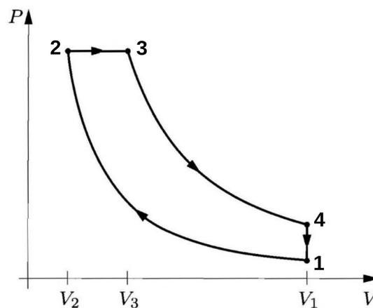
Calculate the efficiency of the Diesel cycle,  $\eta_D$ , in terms of the compression ratio  $r \equiv V_1/V_2 > 1$  and the cutoff ratio  $C \equiv V_3/V_2 > 1$ , where  $C < r$ .
